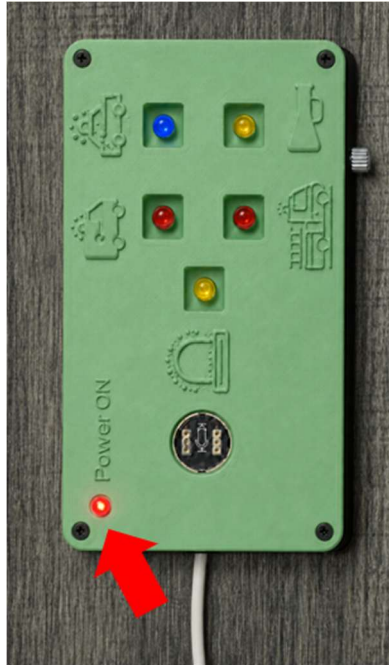
Figure 9. The red arrow points to the system's ON LED indicator. When ON, it will glow Red
