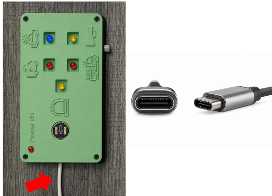
Figure 8. The red arrow points to the system's power input. USB Type-C
