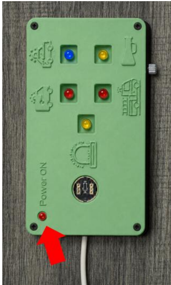
Figure 12. The red arrow points to the system's ON LED indicator. When OFF, it does not glow
