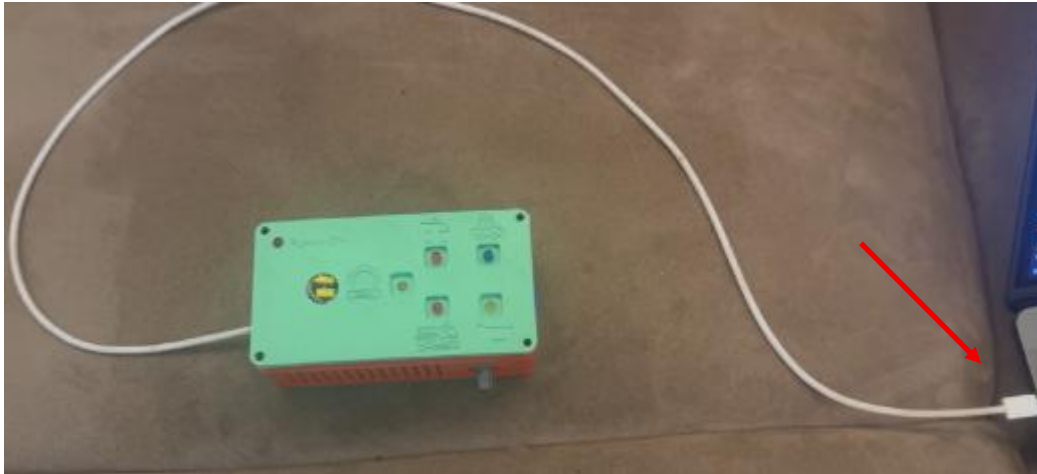
Figure 15. UBS connection to power on.
