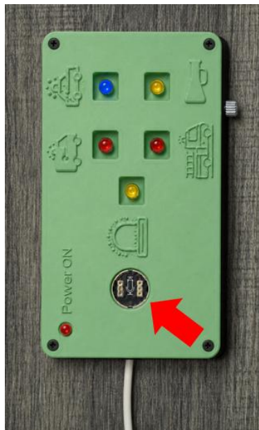
Figure 18. The red arrow points to the system's Sound Sensor
