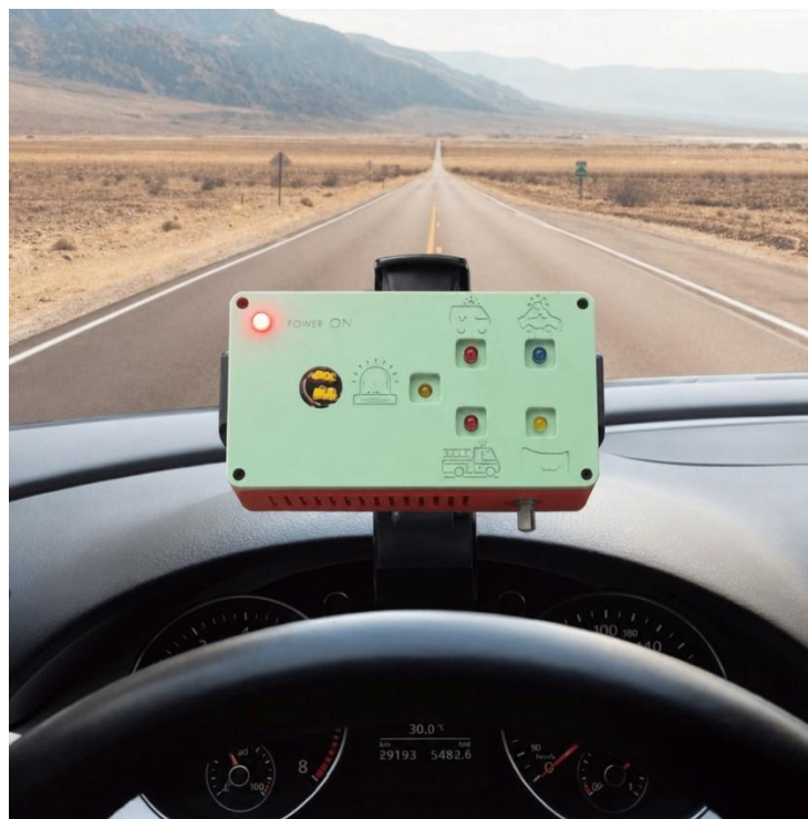
Figure 23. Recommended mounting location directly above the steering wheel for maximum visibility and reduced driver reaction time.
