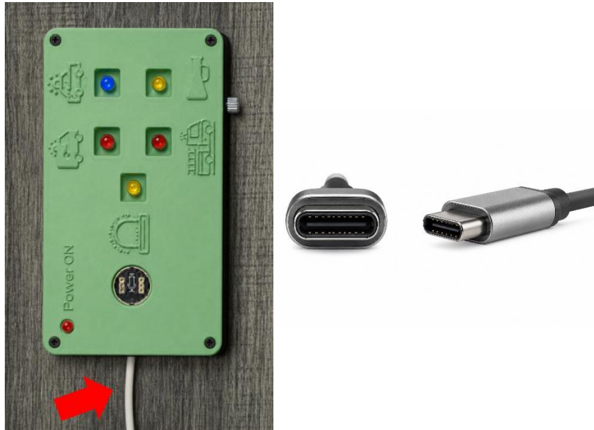
Figure 8. The red arrow points to the system's power input. USB Type-C
